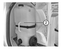
During the trip, the waste water ②tank can be stored in the gasbottle container to save space.
