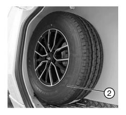
The spare tyre with mount (model/series-specific, optional extra) ② can be stored at the front of the caravan by the gas bottle container. (The mount will only be included in the scope of delivery if the spare tyre is fitted at the factory.)
