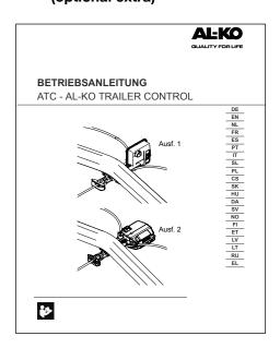
AL-KO Trailer Control (ATC) recognises if the trailer starts to swing too much, beyond the acceptable limits, and reacts automatically. If necessary, the trailer will be braked automatically.
